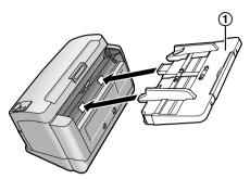
**b.** Push the right (①) and left (②) sides of the feed tray in that order until the feed tray locks in place.
