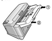
**c.** Pull out the feed extension tray in the direction of the arrow shown in the illustration below.
