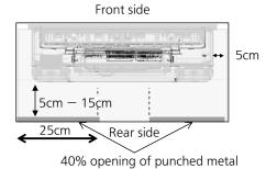
(\*1) When the spacing behind the display exceeds 15cm, exhaust air may not vent smoothly and be drawn into the Display Inlet. To prevent such a situation, a separator material to isolate the intake and exhaust air shall be installed as illustrated.
